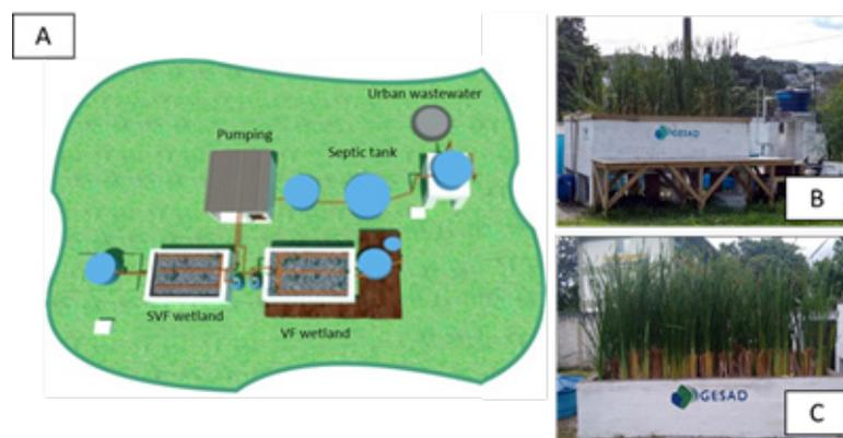
**Figure 1.** Diagram of the treatment plant. (A) Main unit of treatment; (B) Vertical flow CW; (C) Partially saturated vertical flow CW.
