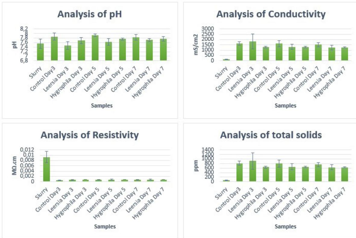
**Figure 1.** Results of the analysis of pH, conductivity, resistivity and total solids, during the hydraulic detention times.
